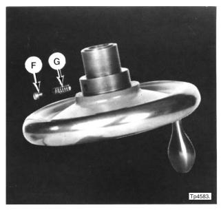
Figure 6.38 - Plug and Spring for Dial
