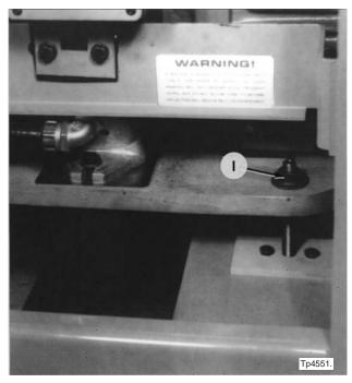
Figure 6.4 - Drive Belt Adjusting Screw
