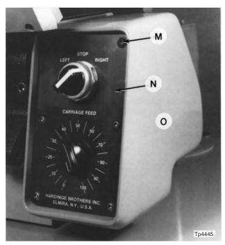
Figure 3.39 - Power Feed Control Box
