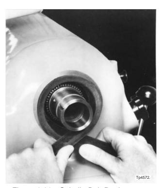
Figure 6.26 - Spindle Belt Replacement
