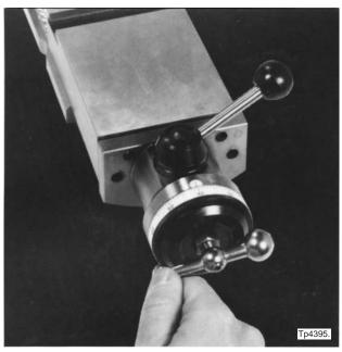
Figure 2.13 - End Cap and Dial Assembly Removal
