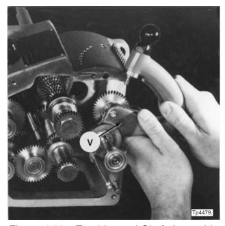
Figure 4.23 - Tumbler and Shaft Assembly Removal
