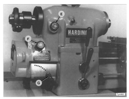
Figure 4.4 - Gearbox (Front View)
