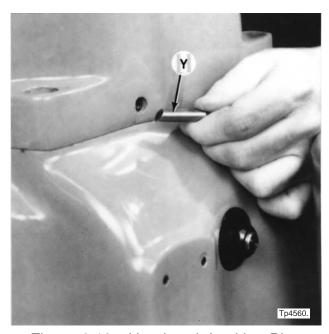
Figure 6.13 - Headstock Locking Plug
