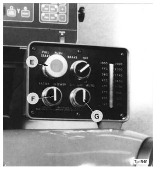
Figure 6.2 - Variable Speed Control Box
