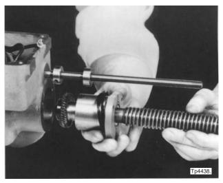
Figure 3.32 - Vertical Feed Screw Removal
