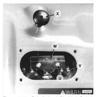
Figure 6.12 - Spindle Lock Pin Limit Switch
