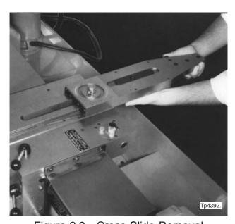
Figure 2.9 - Cross Slide Removal
