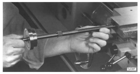
Figure 2.4 - Cross Slide Feed Screw Removal
