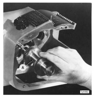
Figure 4.26 - Reverse Shaft Removal
