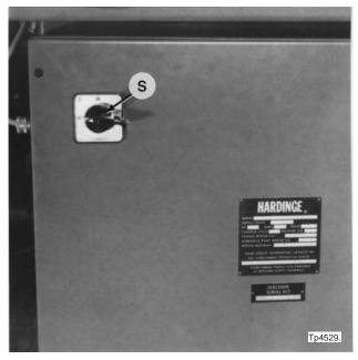
Figure 4.73 - Main Disconnect Switch
