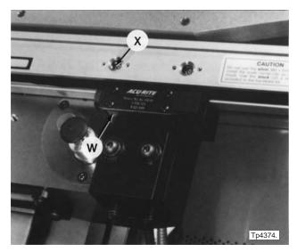
Figure 1.48 - Mounting Holes for Alignment Brackets
