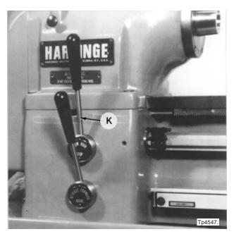
Figure 5.10 - Headstock Levers (TFB®-H Machines)
