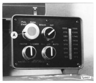
Figure 4.1 - Variable Speed Control Box (HLV®-H Version Shown)
