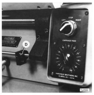
Figure 6.15 - Stop Rod Positive Stop
