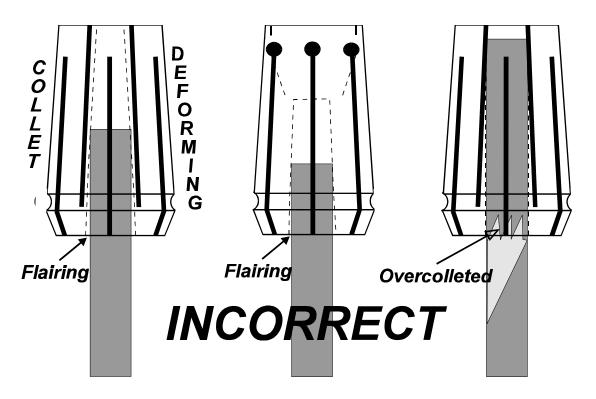
Heat is the biggest enemy of the tool, and the first place the heat goes from the tool is into the collet. It is also important to note that collets are made of spring steel that can, and will over a period of time lose it's elasticity and harden, making it increasingly tougher to tighten adequately. As this hardening takes place, the steel does not fatigue evenly and often causes the collet to grip tighter on one side than the other, creating runout in the tool.
