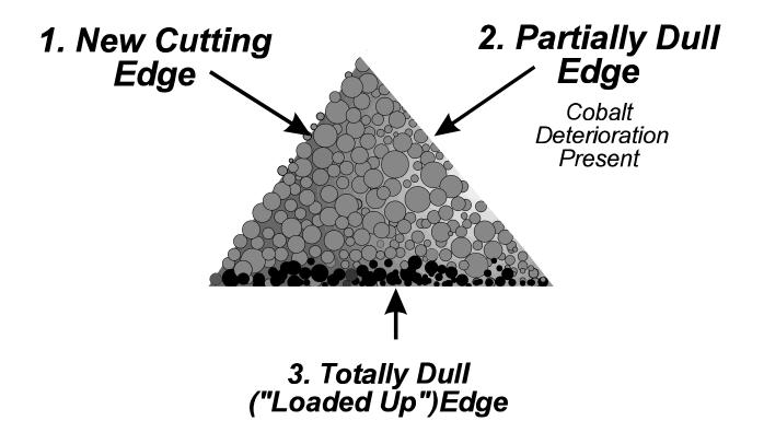
Edge Deterioration due to "Hot Corrosion" of the cobalt binder at the surface of the cutting edge caused by heat generated during the machining process. This "Hot Corrosion" process cannot be stopped!
