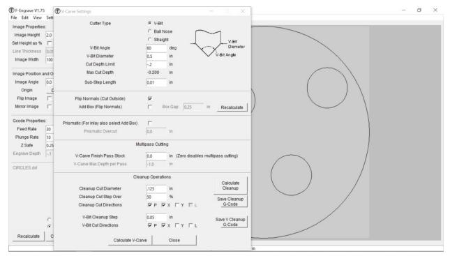
V-bit Angle: 60 degree is what I normally use. 30 degree works for deeper carves.
