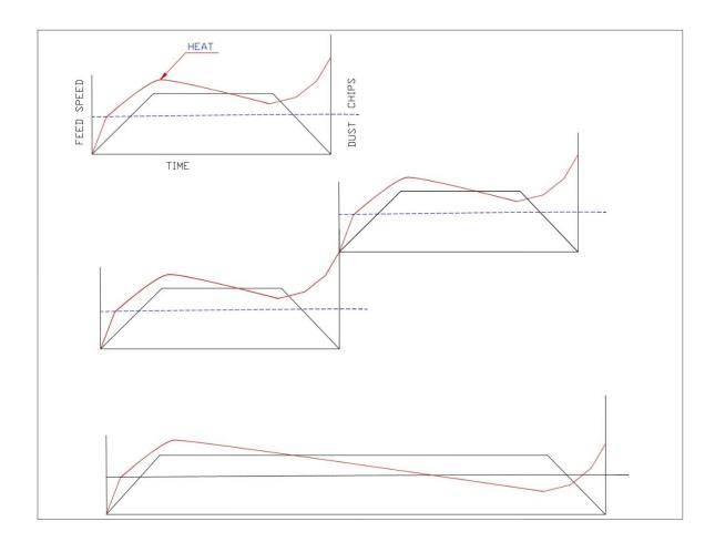
The task then becomes to minimize dust production while maintaining quality of cut. The position of the 'dust to chips' line depends on spindle speed and feed rate. A slower spindle speed or a faster feed rate will lower that line.
